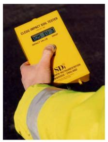
The CIST/882 Readout Unit is held in the hand during testing. It displays readings of Impact Value (IV) and also shows the number of times that the hammer has been dropped during each test operation. Unlike previous models the user does not need to keep the 'On' button pressed during testing.
