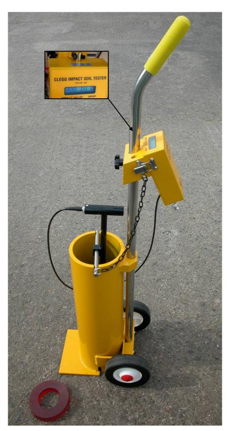
Here the tester may be used in obtaining data for estimating the traffic carrying potential of lightly surfaced low traffic roads.
