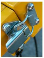
Readout Unit is securely clipped to the Adjustable Readout.
