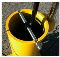
20 Kg Hammer supported by Support Pin during transit.
