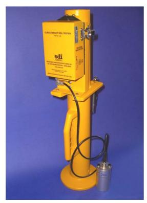
Introduction: - The CIST/883 Golf Course Tester designed and manufactured by SD Instrumentation Ltd provides an easy and straightforward means for measuring the variations in strength on fairways and for helping determine the uniformity of an area. The equipment consists of a two 0.5 Kg hammer probes that operate independently within a vertical guide tube.
