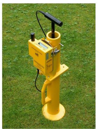
Introduction: - The GPS equipped CIST/884 Clegg Impact Soil Tester manufactured by SDi provides an easy and straightforward means for measuring sports surface firmness using the 2.25 Kg hammer. For golf course testing a 0.5 Kg probe is used instead. The GPS 884 readout is clamped to the guide tube and the displayed reading is viewed from the top during use. Single button operation design provided for easy use.
