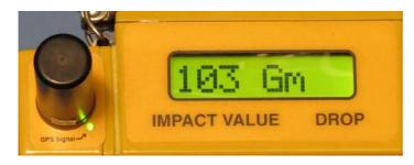
The Readout Unit displays readings of firmness (Gm) on its large easy to see back lit display.
