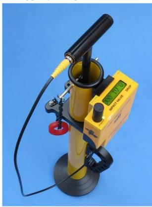
Introduction: - The GPS equipped 4.5 Kg CIST/884 Clegg Impact Soil Tester manufactured by SDi provides an easy and straightforward means for measuring and controlling soil strength and consolidation levels during trench re-instatement. The GPS 884 readout is held to the Bumble Bee guide tube and the displayed reading is viewed from the top during use. Single button operation design provided for easy use.
